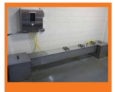
The **SUNLIGHT H-4XE-HO** is a sixteen (16) lamp biologically validated low pressure high output UV disinfection channel system that treats 1 MGD (for a 200/100 ml) and is designed to treat a 12" water level .
